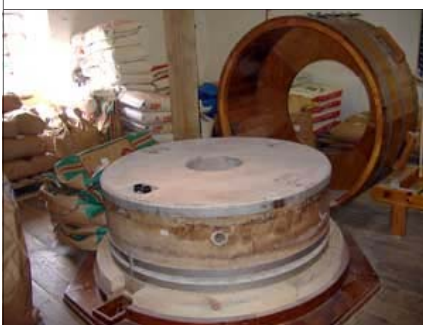
The new millstones in working position, with old the tun to the rear
