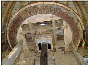
Thrigby— brakewheel & wind shaft
